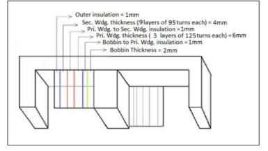
Fig 1 Winding arrangement of 100 VA, 50 Hz Transformer
